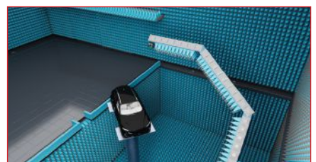
▲ Fig. 4 Full-vehicle OTA anechoic test environment.
