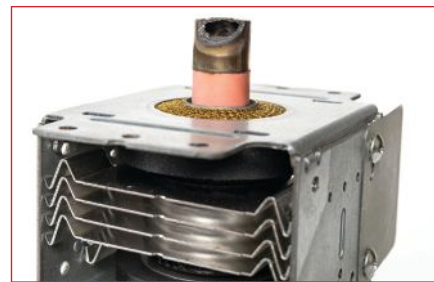
▲ Fig. 4 High voltage magnetron failure.
