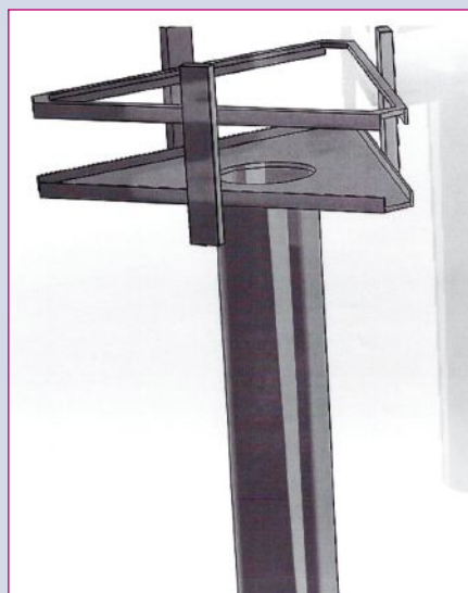
▲ Fig. 10 Mounting configuration for three-sector base station.
