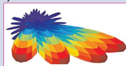
▲ Fig. 3 Rendering of a simple four-beam azimuth pattern.
