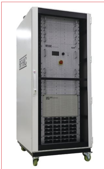
▲ Fig. 1 RFHIC RIK0930K-40TG 30 kW system.
