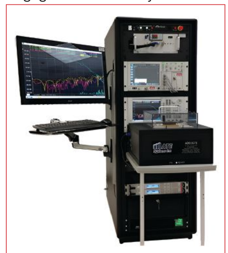
▲ Fig. 5 Automated test rack and fixture with robotic handling and interconnect. Source: ATE Systems Inc.
