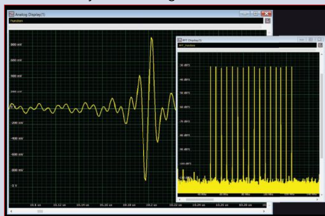
▲ Fig. 1 16 superimposed sine waves and the FFT.
